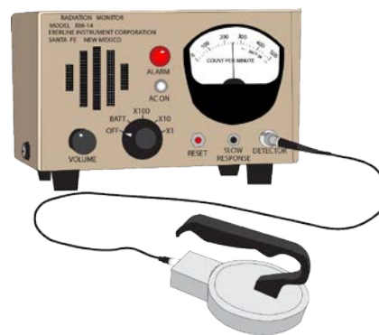
Friskers are one tool used to measure contamination.
