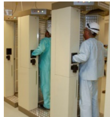
Personnel checking for contamination with PCMs.
